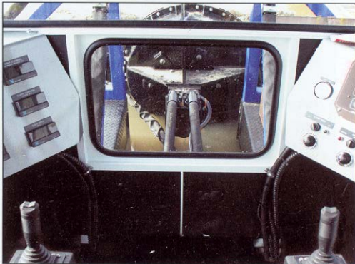
All Versi-Dredge® models come standard with joystick controls and digital gauges for ease of operation.
