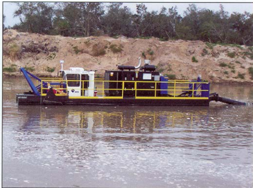
A Model 7012 HP removes sand from a sand mine in Eastern Florida.
